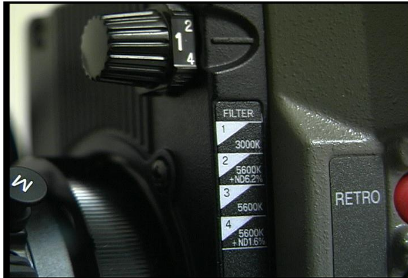
Figure 2-10, Filter wheel found on the Ikegami 201W ENG Camera.
