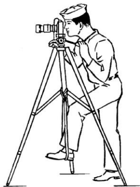
Using a foot strap to make a tripod more rigid
